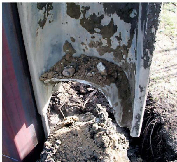
**Figure 2.3:** Damaged sheet pile, from Viking and Garcia Benito [6]. Photo: Viking K. Example of local axial buckling and material fracture due to round boulder encountered.
