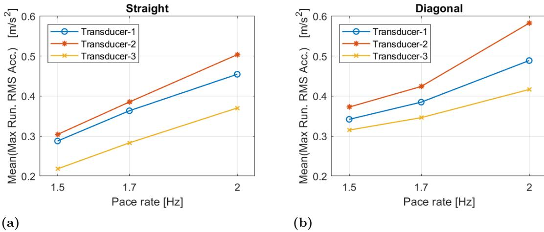
**Figure 4.5:** Mean of the maximum Running RMS for all test persons (a) Straight path (b) Diagonal path
