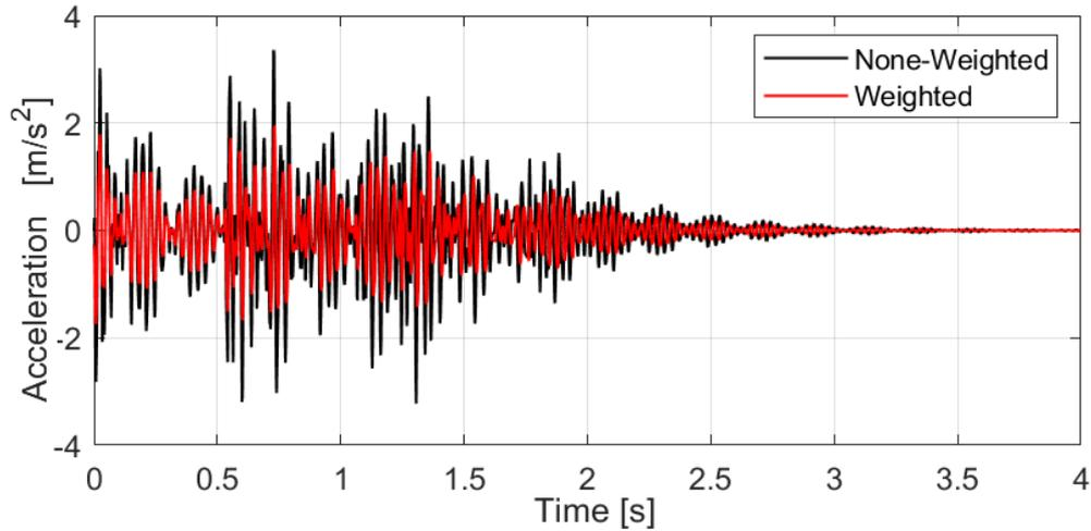
**Figure 5.4:** The weighed and non-weighted signal, respectively for the simulation in Transducer-2 when using the pace rate 2.0 Hz
