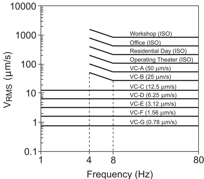
**Figure 2.2:** VC curves for sensitive equipment, compared against ISO-criteria for human perception. Figure used with permission from [14]
