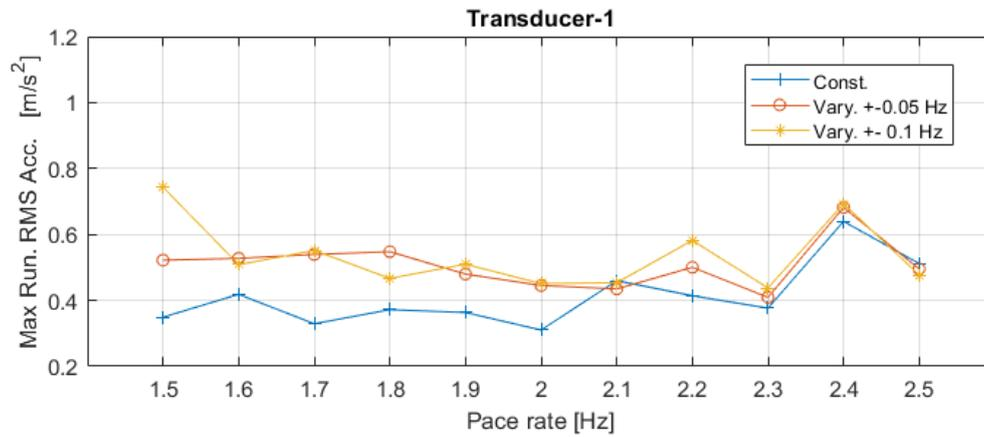
**Figure B.1:** Response in Transducer-1 when the pedestrian has a constant pace rate and when the pace rate varies with  $\pm 0.05$  Hz respectively  $\pm 0.1$  Hz. The variation is relative to the second step which has a pace rate according to the x-axis
