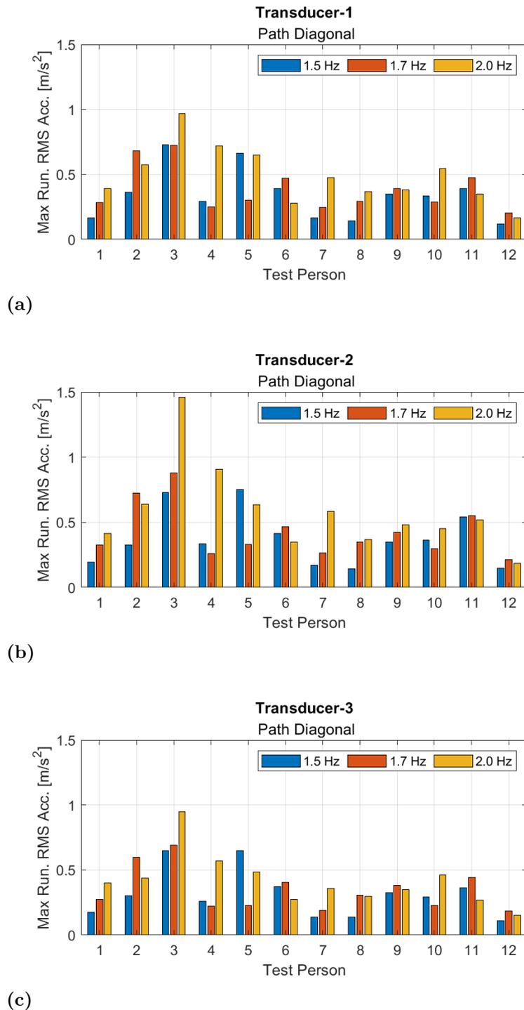
**Figure 4.4:** The maximum 1 second Running RMS when walking along the diagonal path for the different persons (a) Transducer-1 (b) Transducer-2 (c) Transducer-3
