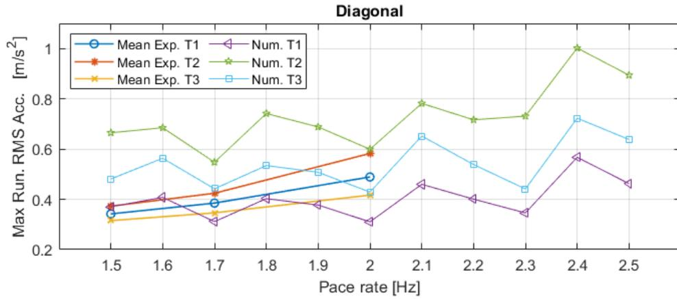
**Figure 5.6:** The maximum RMS for the numerical simulations compared against the mean value from the experimental measurements
