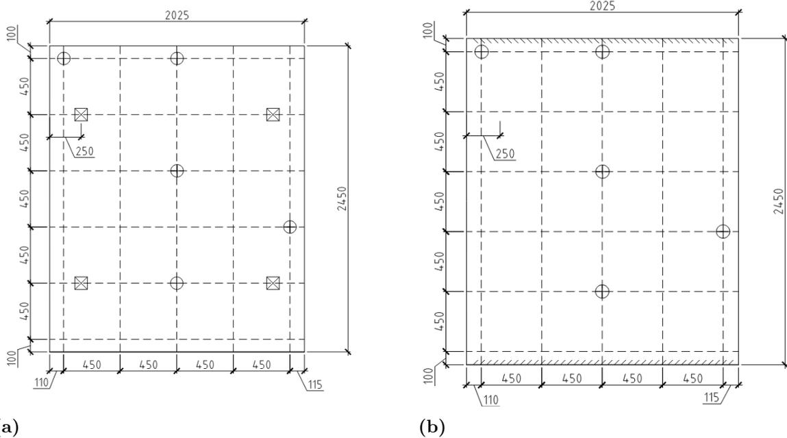
**Figure 3.4:** (a) Measurement grid and position of the supports for the floor when resting on air cushions. Intersection of the dashed lines marks impact points, circle marks accelerometer and square supports (b) Measurement grid and position of the supports for the floor when resting on two LWL beams. Intersection of the dashed lines marks impact points, circle marks accelerometer and hatched lines supports
