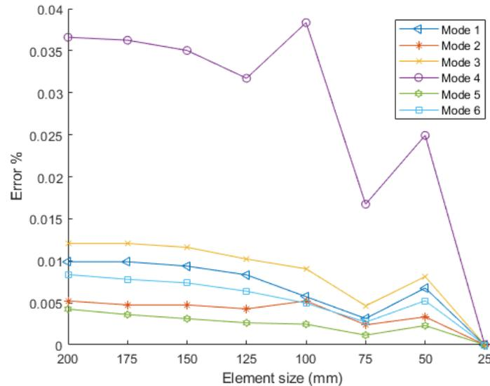
**Figure 3.3:** Convergence study for the floor when changing the element size in the plane of the floor
