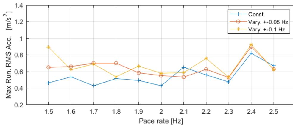
**Figure B.2:** Response in Transducer-3 when the pedestrian has a constant pace rate and when the pace rate varies with  $\pm 0.05$  Hz respectively  $\pm 0.1$  Hz. The variation is relative to the second step which has a pace rate according to the x-axis
