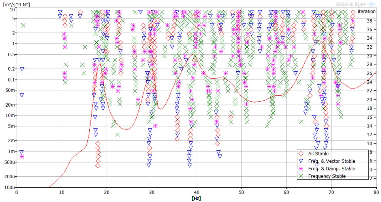
**Figure 3.9:** Mean frequency response function and stabilization plot when the floor was supported by two LVL beams
