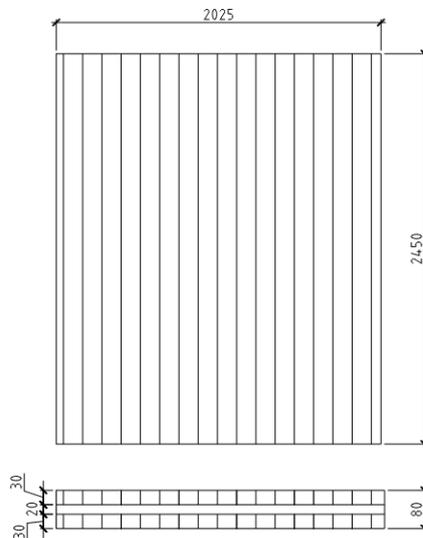
**Figure 3.1:** The CLT floor used for measurements
