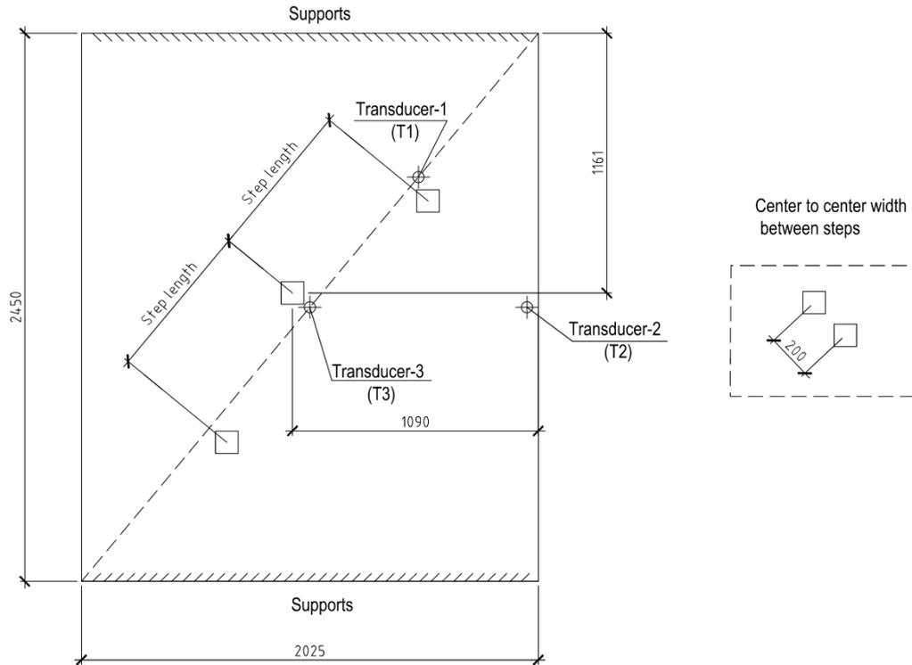
**Figure 5.2:** Illustrates how the load was applied in each of the three steps. The centre step was stationary while the position of the two other was changed as a function of the pace rate
