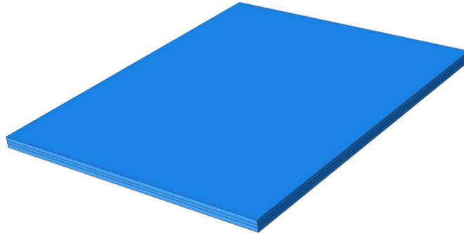
**Figure 3.2:** Model in Abaqus based on solid elements
