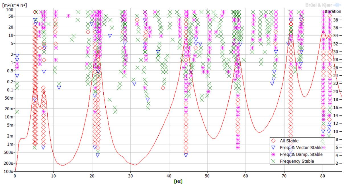
**Figure 3.6:** Mean frequency response function and stabilization plot when the floor was supported by air pillows
