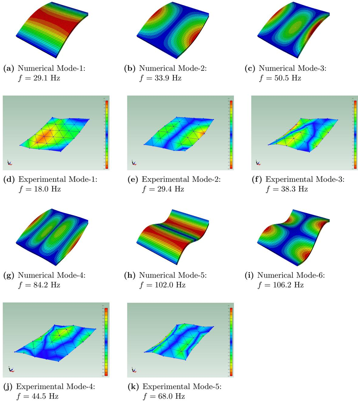
**Figure 3.10:** First five and six modes for the experimental measurement, respectively the numeral simulation, when the floor was supported by two LVL beams.
