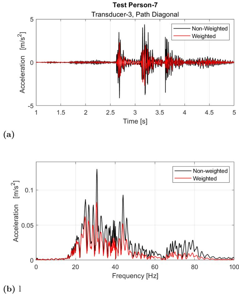
**Figure 4.2:** (a) Frequency weighted and non-frequency weighted response, respectively in Transducer-2 for Person-7 when walking along the diagonal path with the pace rate 2.0 Hz (b) FFT of the weighted respectively the non-weighted signal, respectively
