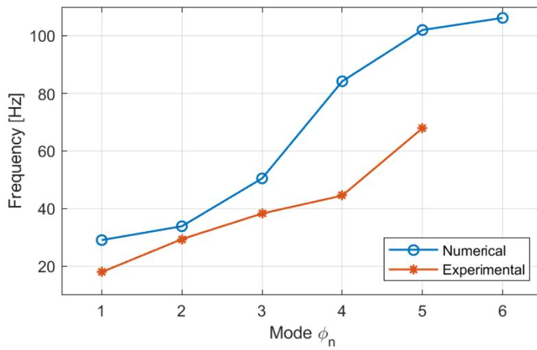
**Figure 3.11:** The natural frequencies for the numerical simulation and experimental measurement, respectively when the floor was supported by two LVL beams
