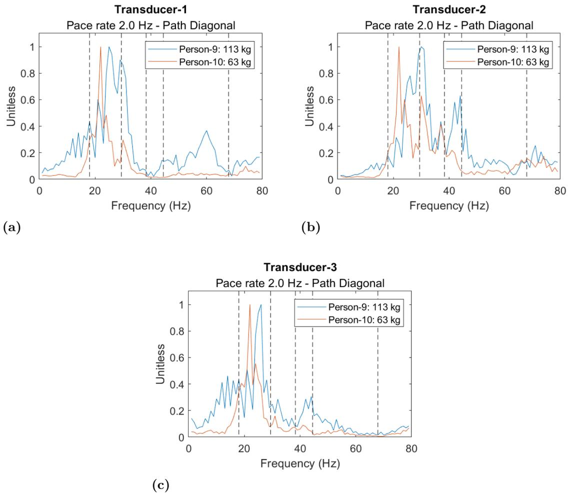
**Figure 4.7:** Comparison of how the weight affects the dynamic properties of the floor. The dashed line represents the natural frequencies
