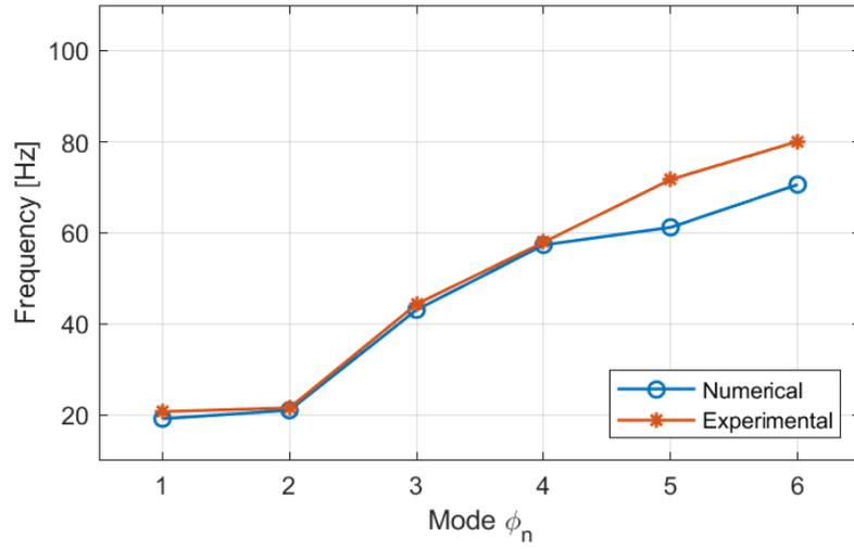
**Figure 3.8:** The natural frequencies for the numerical simulation and experimental measurement, respectively when the floor was supported by four air cushions
