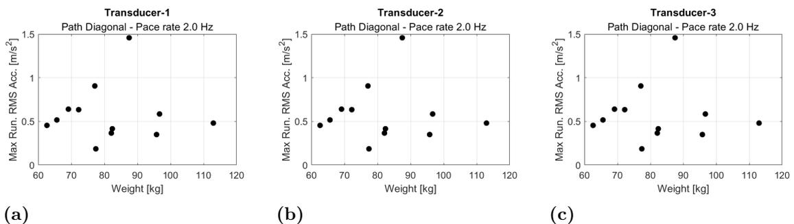
**Figure 4.8:** The response normalized to the body weight 80 kg, plotted against the test persons mas
