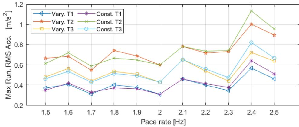
**Figure 5.7:** Varying striding length compared against a constant length of 0.8 meter
