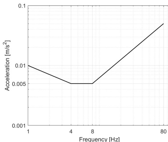
**Figure 2.1:** Base curve for human perception according to ISO-2631-1:1997 and ISO 10137:2008
