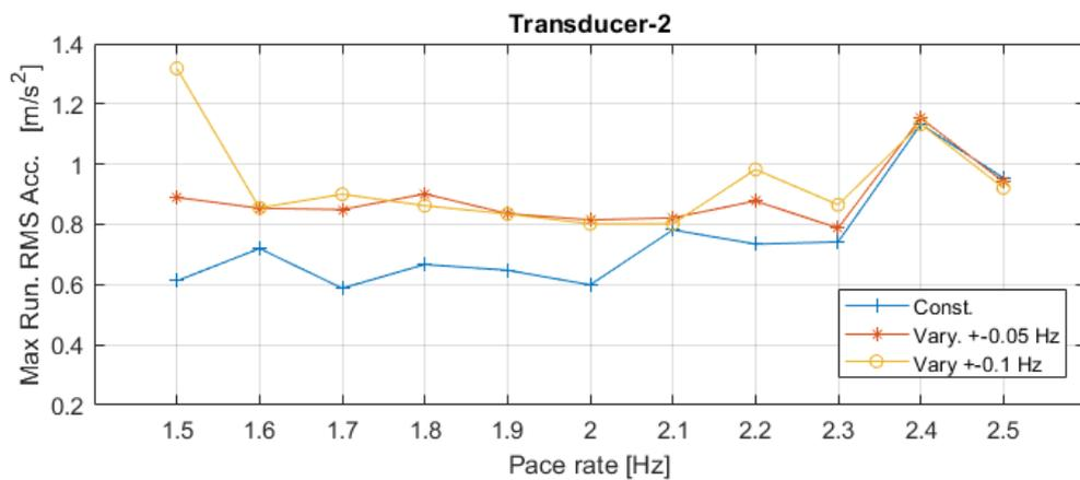
**Figure 5.8:** Response in Transducer-2 when the pedestrian has a constant pace rate and when the pace rate varies with  $\pm 0.05$  Hz respectively  $\pm 0.1$  Hz. The variation is relative to the second step which has a pace rate according to the x-axis
