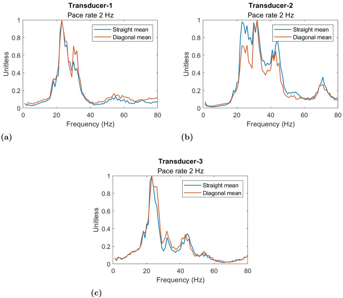
**Figure 4.6:** Overlapped response processed into 1 Hz bands, when walking along the straight and the diagonal path for the pacing rate 2.0 Hz. The amplitudes between the diagonal and the straight path is not comparable, due to different signal lengths
