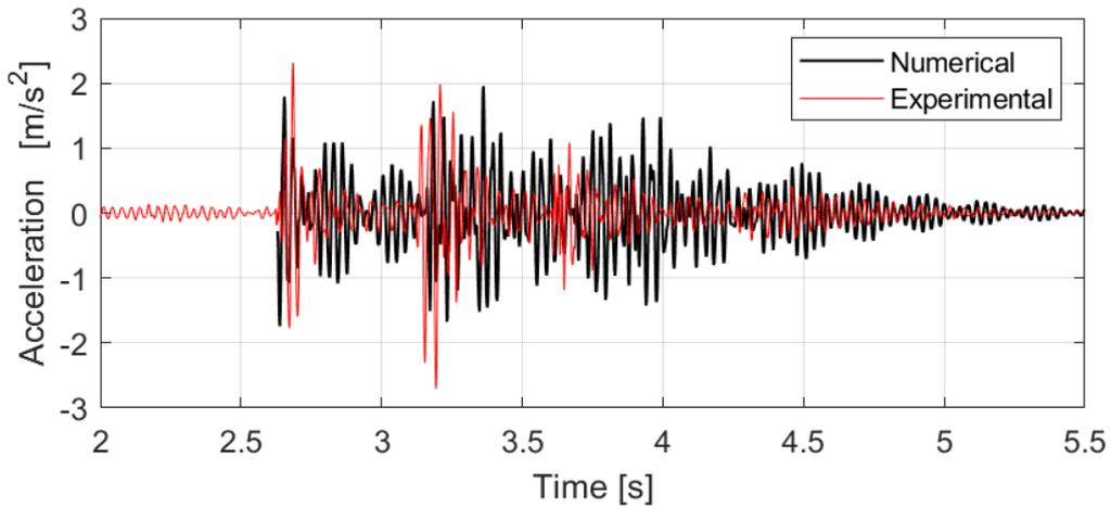
**Figure 5.5:** The response in Transducer-2 from Person-7 walking with the pace rate 2.0 Hz compared against corresponding simulation, shifted with 2.6 seconds
