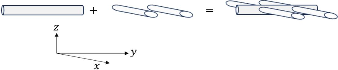
**Figure 5.3:** Schematic view of the assumption of having reinforcement in the same plane
