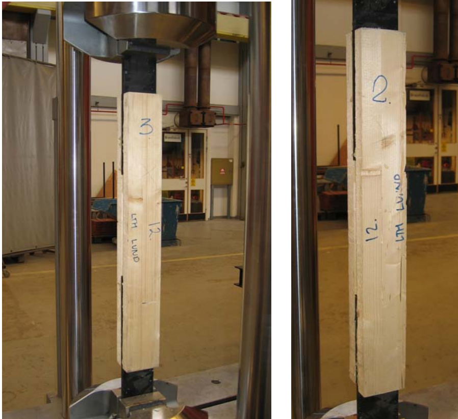
Series 12, inner steel plate rubber foil lap joints, 160 mm
