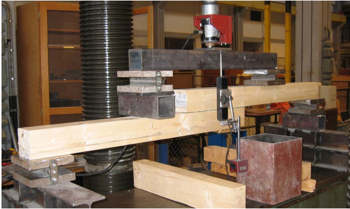
Series 1a, single lap joint in flatwise bending
