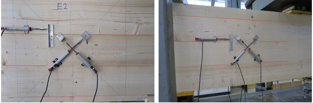
**Figure 34:** Placement of potentiometers for E2 (left) and E3 (right) in relation to placement of longitudinal laminations.
