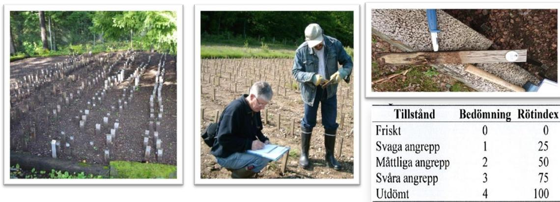
Figure 14. Field test according to EN 252.
