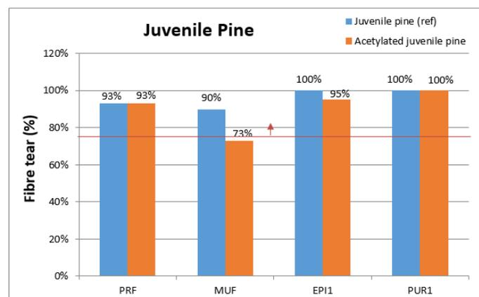
Figure 20. Fibre tear (%) for each investigated adhesive system glued on acetylated juvenile pine (orange) and reference juvenile pine (blue). Internal requirement >75%.
