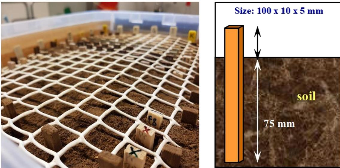
Figure 11. Test set -up for ENV 807.
