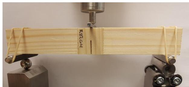
*Figure 26. Three-point SENB specimen used for determination of specific fracture energy.*
