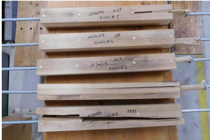
Figure 40. Failure mode for acetylated Birch samples.
