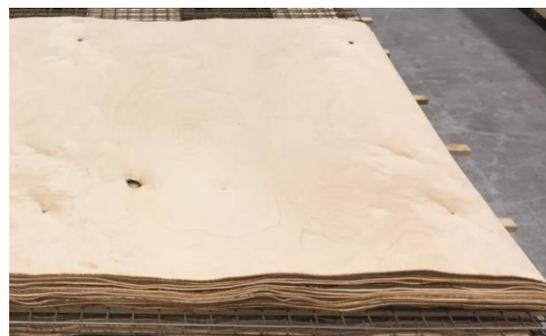
*Figure 3. Birch veneers used for acetylation.*
