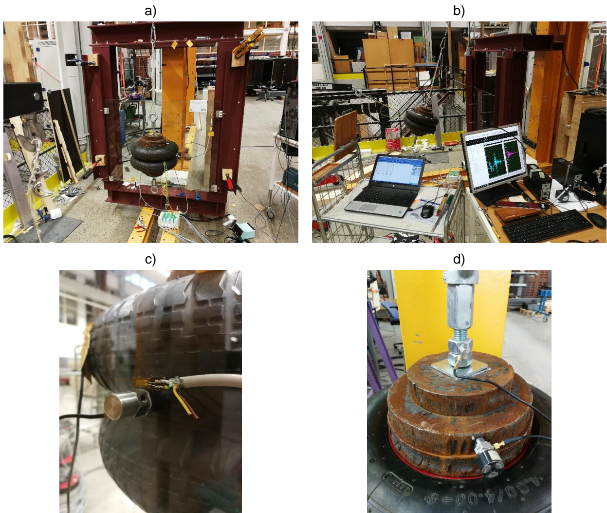
Fig. 2 Soft-body impact test set-up: a) steel rig, b) computers logging data from strain gauges and accelerometers, c) strain gauge and accelerometer mounted to the glass specimen, d) accelerometer mounted to the impactor.
