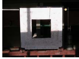
Figure. 4.3 Infill wall with 60% central opening before loading
