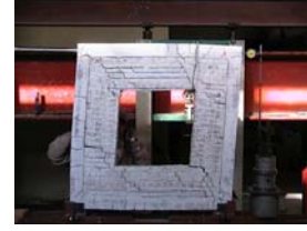
Figure. 4.4 Infill wall with 60% central opening after loading
